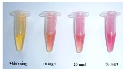
**2. Test of effluent from fish:** Add 1.5 ml of effluent and 1 cm of test strip into Eppendorf tube. Waite 2 minutes. The appearance of pink or pink-orange color is indication of urea.
