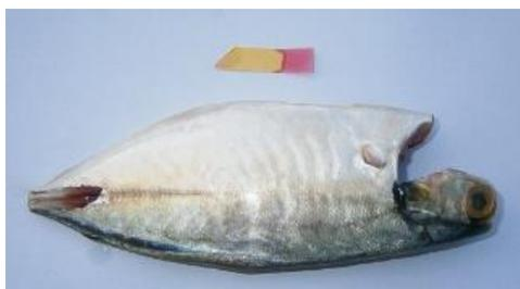
**1. Test directly on fish skin:** press a test strip on wet fish, so that the strip became wet. Waite 2 minutes. The appearance of pink or pink-orange color is indication of urea.
